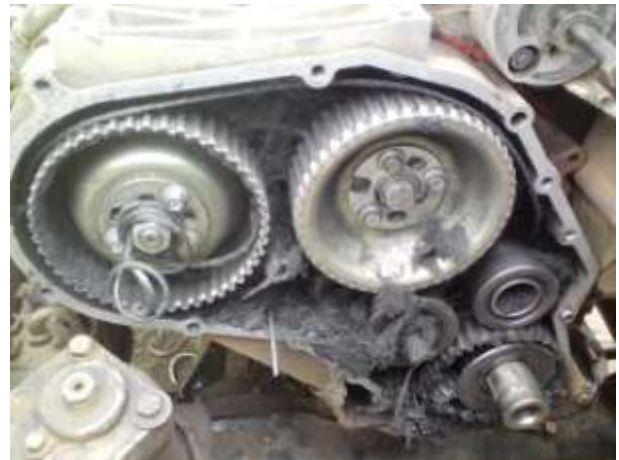
Picture 6: Shredded timing belt on our trusty Land Rover
